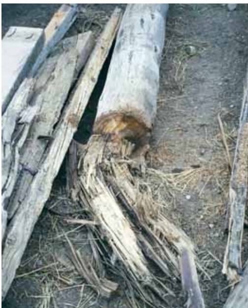
Pilings pulled from the canal after the incident showed the timbers had completely rotted below the water level.
