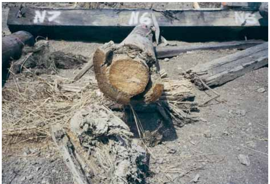
Pilings pulled from the canal after the incident showed the timbers had completely rotted below the water level.
