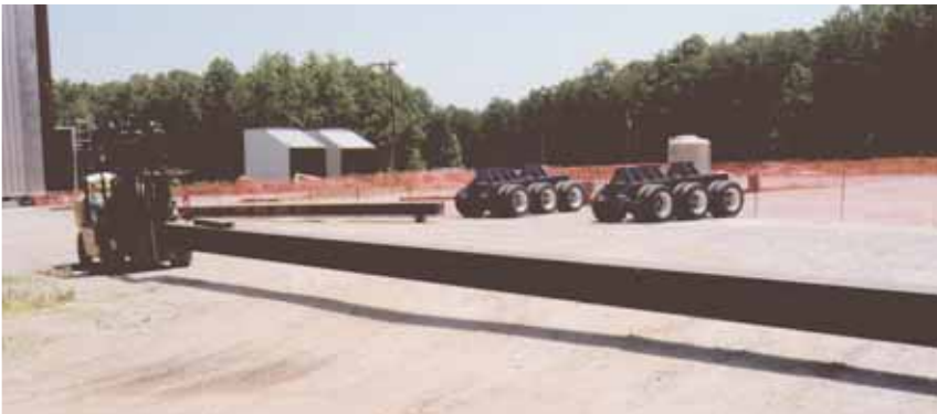
This Beam Dolly is used to facilitate movement of large beams during setup.
