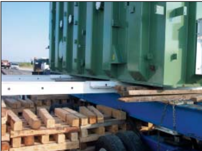
Transformer being transferred from the railcar to Minty's transporter.
