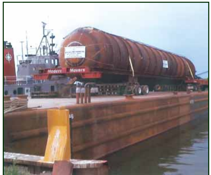
Loaded, blocked and secured on the barge in Sandusky, ready for the two-week trip through the Great Lakes
