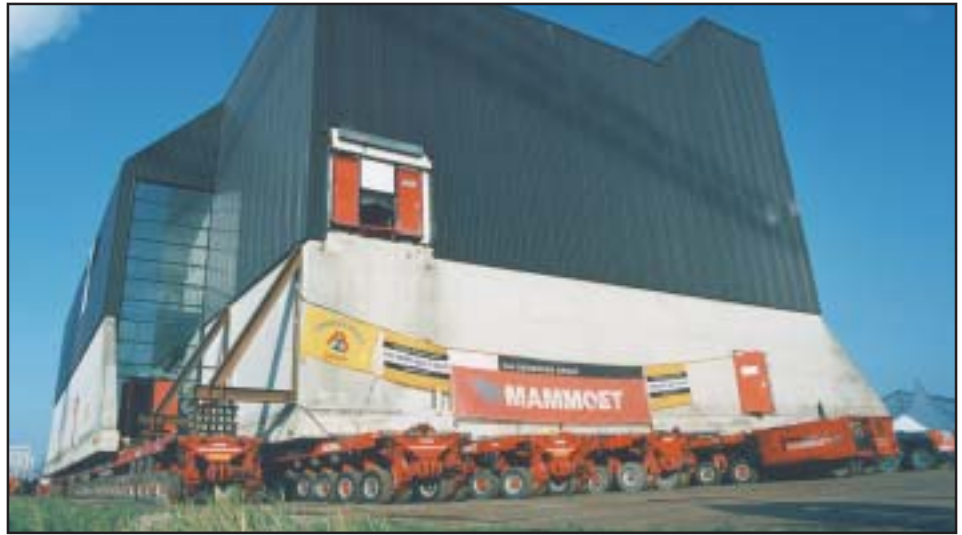
A 90-degree turn was successfully rounded guided by the linked-up computers of all seven transporters, steering the axles in the correct radius.
