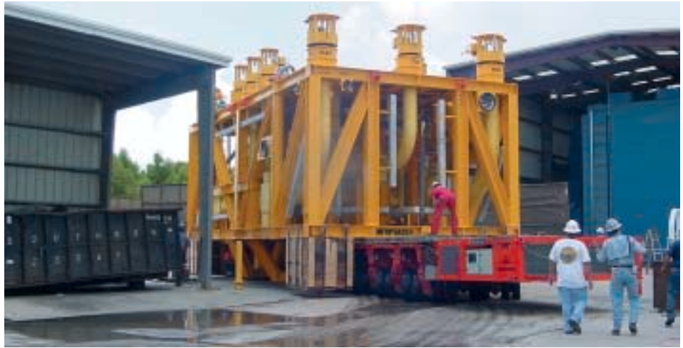
A 250 ton jacket is rotated through 90-degrees on a set two 14-line Goldhofers.
