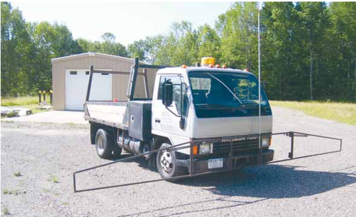
Swinging gate we fabricated to survey the route, height of wires and width of structure
