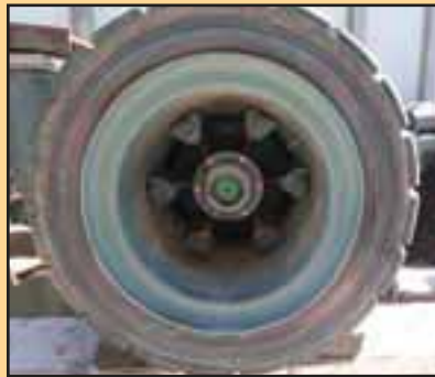
NEW TIRES: 24 ply, 12 inches wide, 28 inches tall, load capacity, each, static: 15,399 lbs
